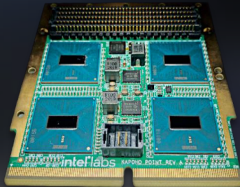
Kapoho Point Stackable 8-chip board
